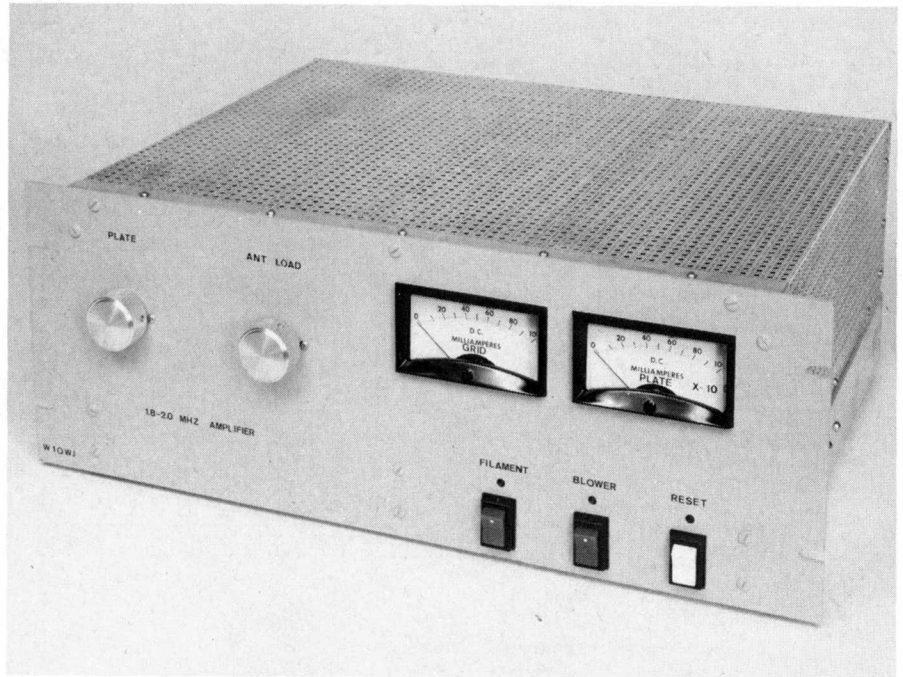
Fig. 51 — The 160-meter amplifier is built behind a 19- × 7-inch rack panel. Meters with bezels add to the clean appearance of the unit.
