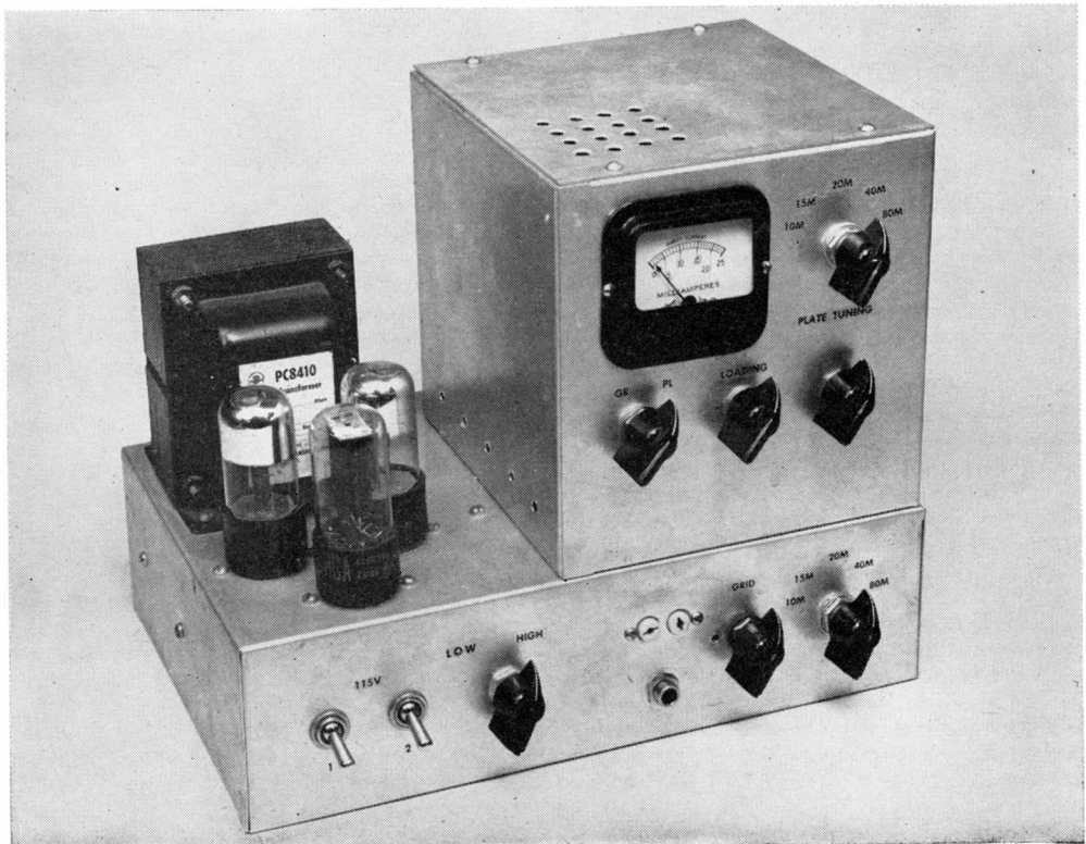
Fig. 6-64—The base for the 6146 amplifier is a 11 × 7 × 3-inch aluminum chassis. A 6 × 6 × 6-inch aluminum box encloses the amplifier tube and its output circuit. S_2 is to the right of the meter. Below, from left to right, are controls for S_3 , C_7 and C_4 . On the chassis, from left to right, are the power-supply switches (see Fig. 6-66), J_1 (see text) and J_3 , and controls for C_1 and S_1 . Ventilation holes are drilled in the cover in the area above the tube, and along the sides of the box, near the bottom. The power-supply diagram is shown in Fig. 6-66.
